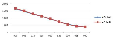
•Smallest TN reads almost same, regardless of whether it is fastened with metal bolt in two holes (located at both ends) or not. Though RF interference is minimal with metal bolts, however, RFcamp recommends not using metal bolts, but 3M 300LSE adhesive or glue for maintaining optimum read performance.
