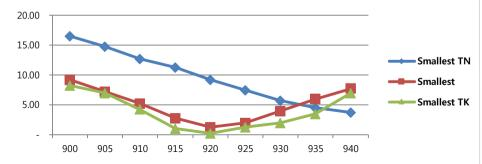
•Smallest TN reads up to 1.5 meters on metal, 25% shorter than Smallest and 60% shorter than Smallest TK.
